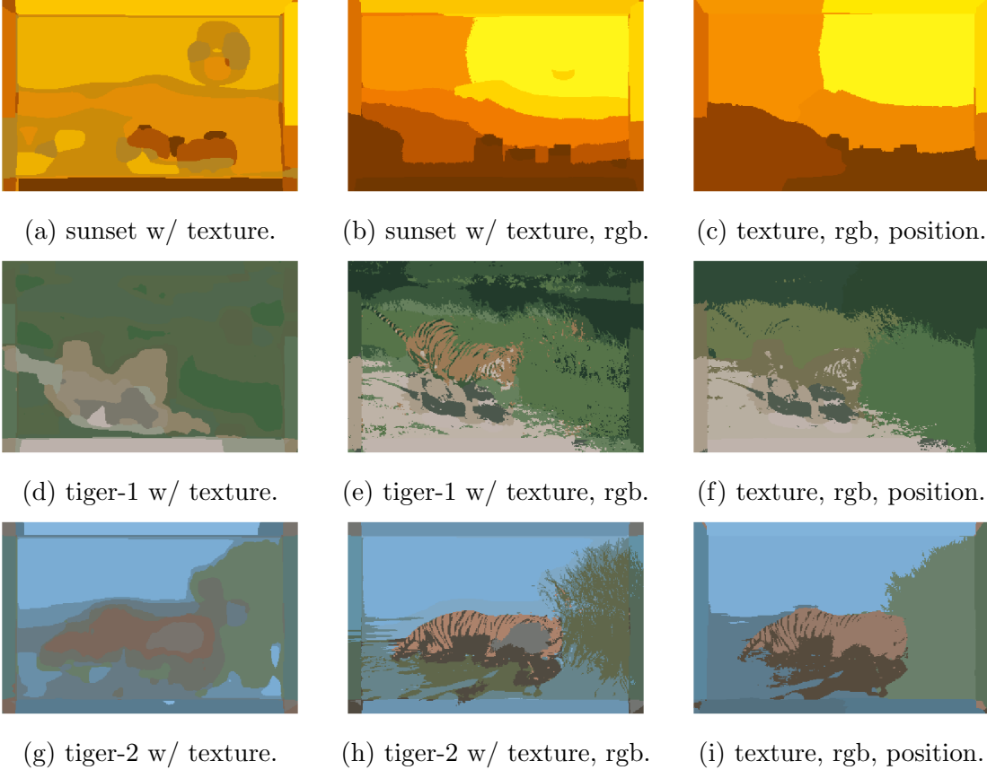
Figure 5: Segmentation of images ( K=10 ) with 5-dimensional feature vector.
